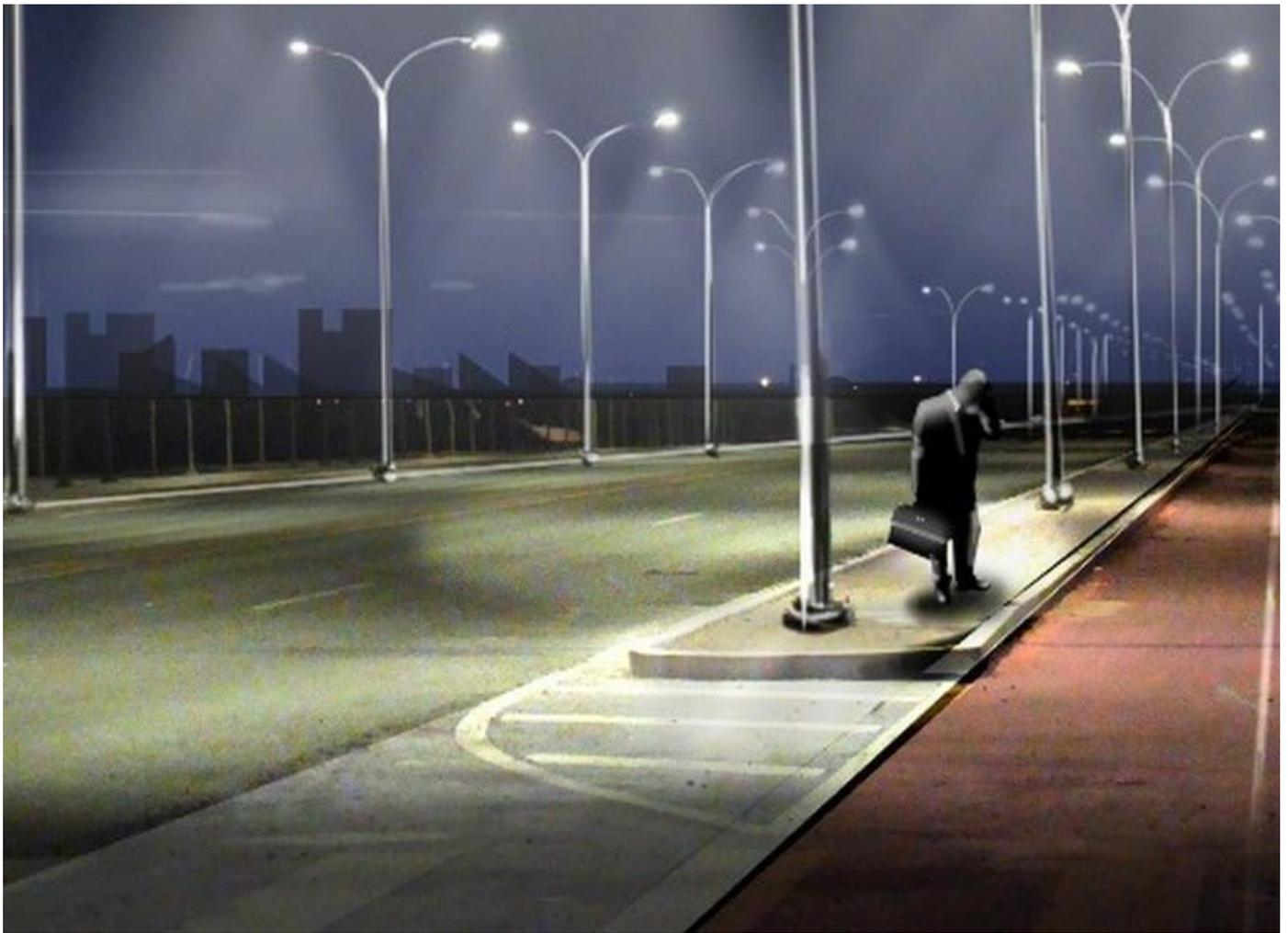
Twilight, which automatically dials down the brightness when no one is around and restores maximum radiance upon detecting the presence of oncoming human activity, has been installed in cities in Holland and Ireland. (Twilight Systems)
