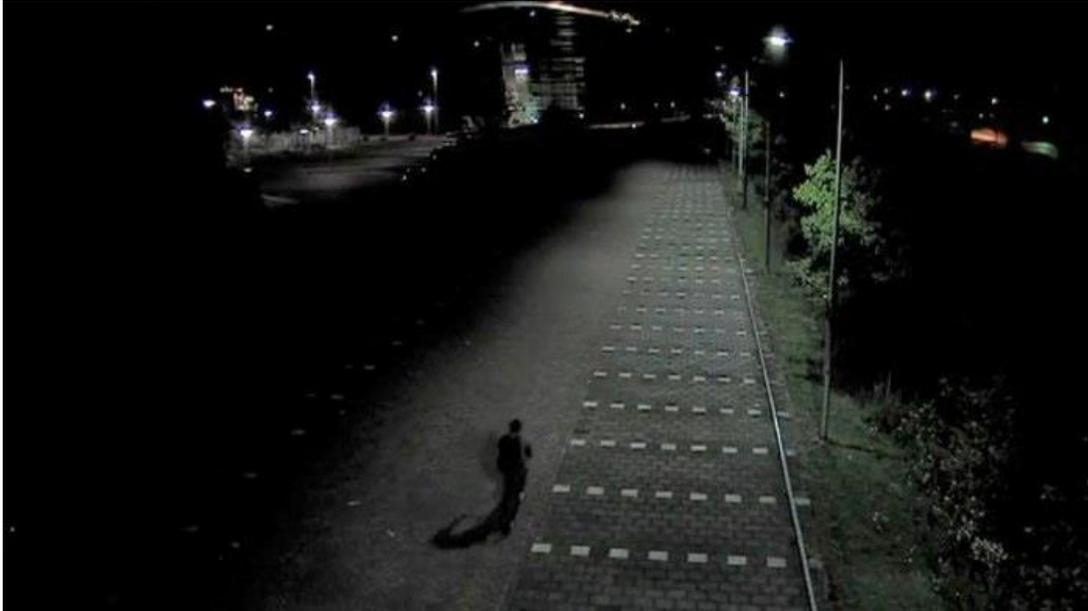
An experimental energy-saving streetlight system automatically dims the lights when no people or moving vehicles are in the area (Image: TU Delft) .
