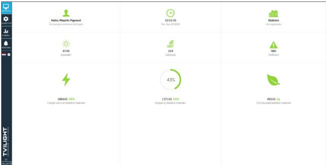
The dashboard in the portal shows that dimming has saved 137,000 kWh over the last six months.
