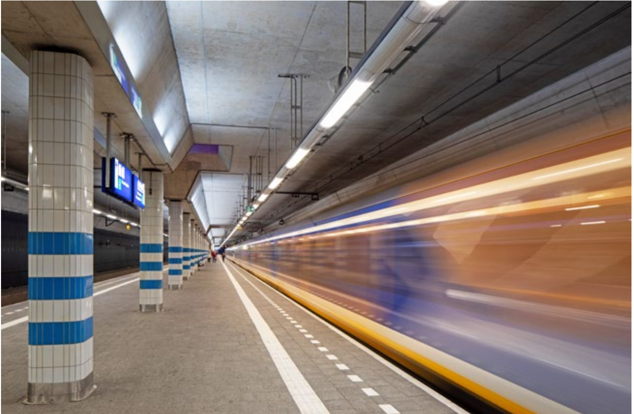
Rijswijk station with 3000K downlighters and 4000K uplighters.
