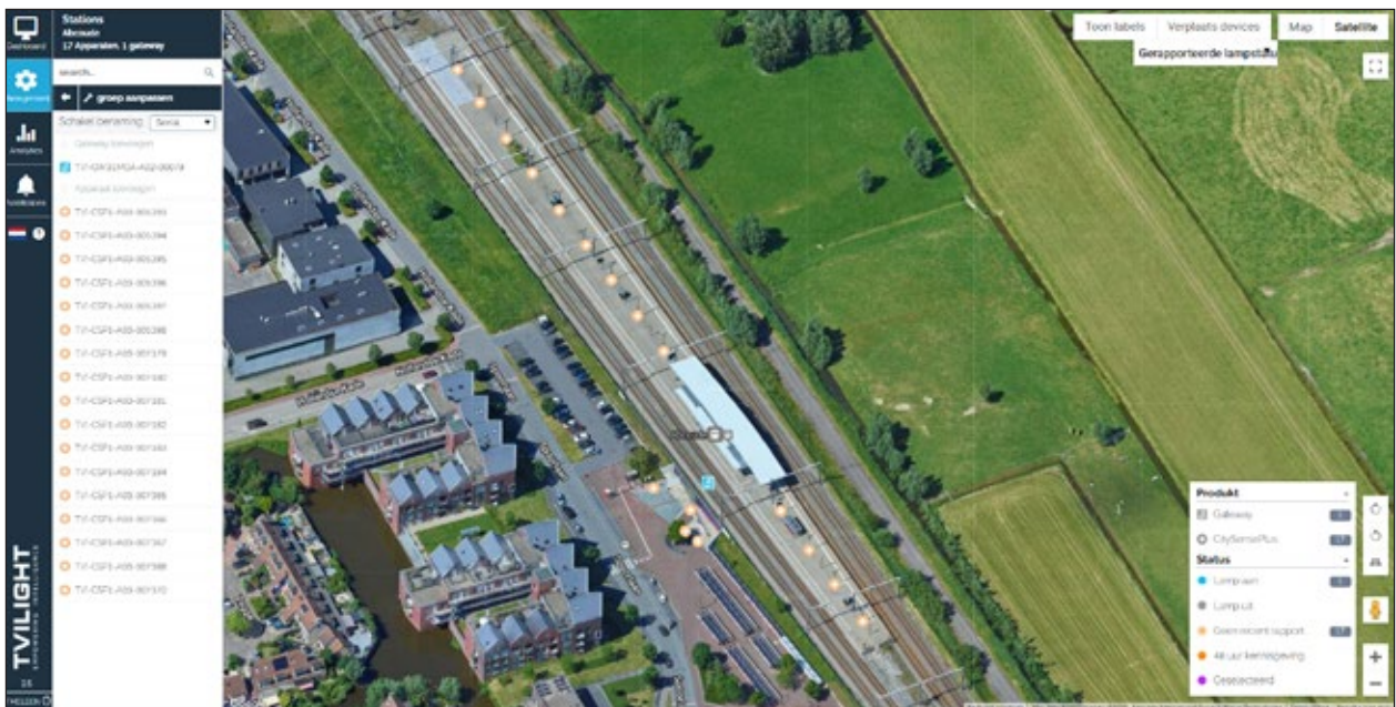
The sensors and Gateway as they appear in the portal at Abcoude station.
